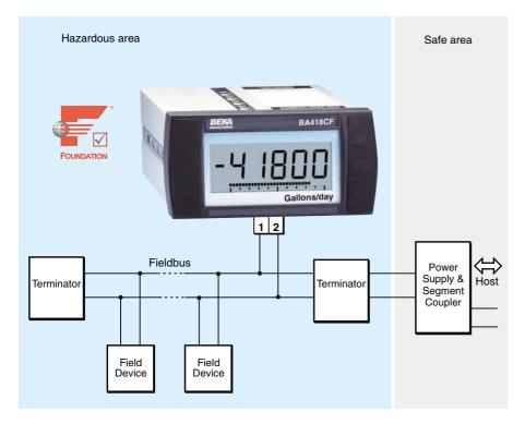
The BA418CF-F Fieldbus Indicator is a new cost-effective intrinsically safe panel mounting instrument that displays a single fieldbus process variable in a hazardous area. Housed in a robust panel mounting enclosure with an IP66 front, the instrument has a large, high contrast five digit display and a horizontal bargraph. The BA418CF-F indicator uses the same technology and compliments the well established BEKA eight variable fieldbus displays that are now in worldwide use.
